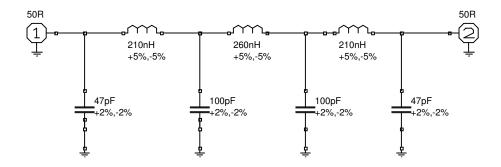
210nH = 6 turns, 6mm air, 0.8mm 260nH = 7 turns, 6mm air, 0.8mm
